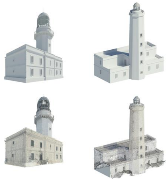
Figure 6: Overlap between parametric model and point cloud
